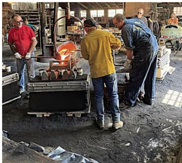
John Henry MacDonald from Nevada Northern Railway pouring one of his grates with Robin Peters and Steve Davies slagging.
